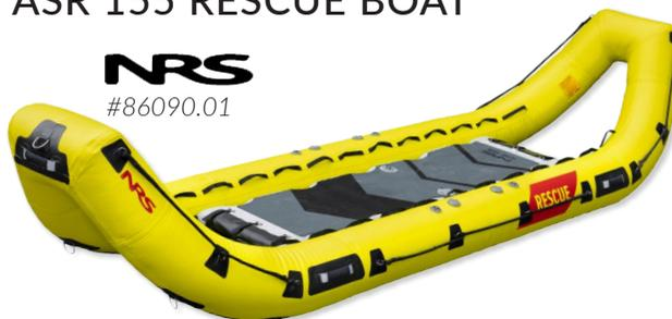
On water, ice or snow the NRS ASR (All Surface Rescue) 155 Rescue Boat puts your rescue team where it needs to be. Overall dimensions (15.5'L x 49"W) deliver the length for carrying 3-4 people and the width for reliable stability in turbulent waters.
