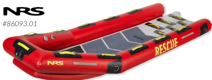
The NRS X-Sled 115 Rescue Boat gives rescuers the options needed for swiftwater, ice, low-head dam and floodwater rescues. Designed to accommodate two rescuers and one victim but can easily float 4-5 people.
