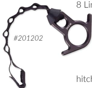
8 Link allows you to extend your Figure 8 descender further away from your harness to make room for a backup Prusik hitch below the descender. It attaches to the Figure 8 with a girth hitch. Multiple carabiner slots allow proper length adjustment.
